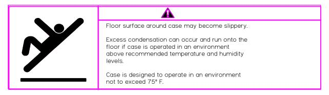
This label is located on the back of the display case.
