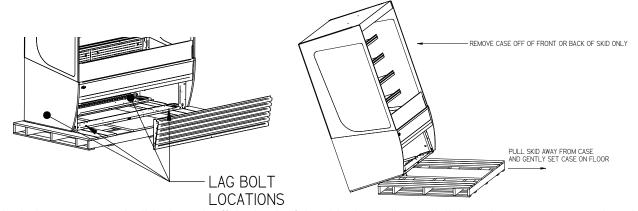
Once all the bolts are removed, slide the unit off the back of the shipping pallet, and tilt it so the rear corner touches the ground. Then have someone move pallet out from under the case and gently tilt the case forward until it touches the floor.
